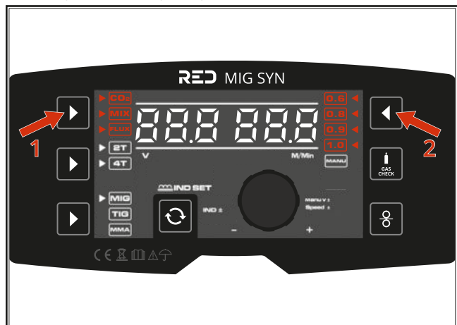
Fig. 10: Setting the welding program
