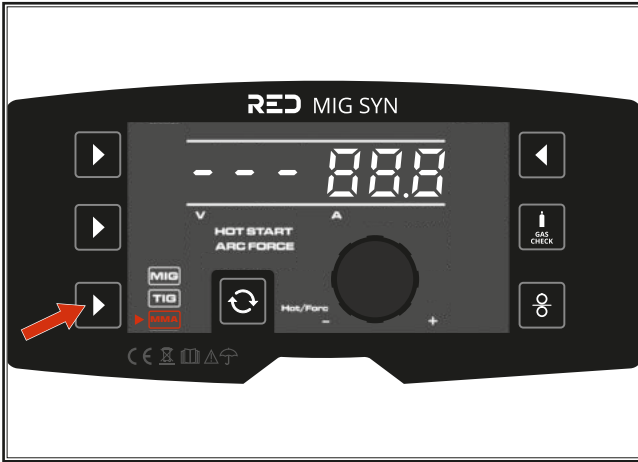
Fig. 21: Setting the welding process
